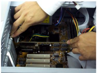
Make sure that the card is pressed evenly and completely into the socket.
